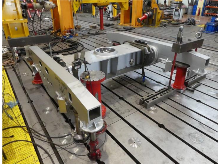
Realisation of torsion stiffness measurement
