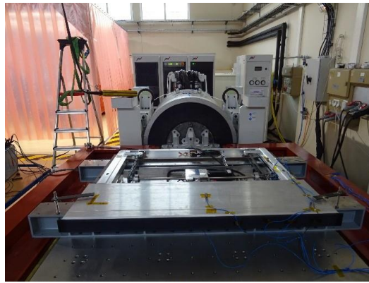
Bridging plate on the vibration test bench
