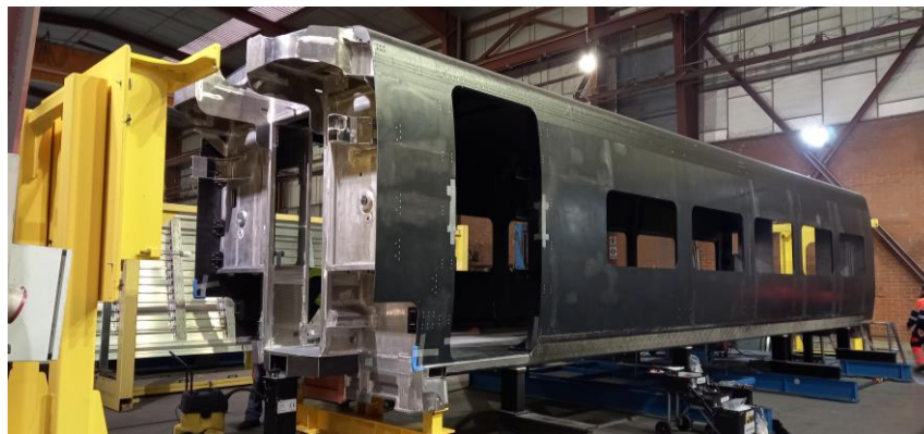
CFRP HS Carbody on the integration tool
